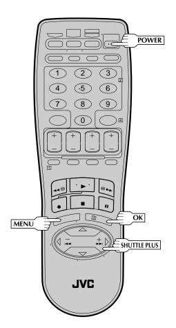
Perform clock setting only if the clock has not been set correctly by the Plug & Play function or you use a cable box. Access the Clock Set screen to perform the Semi-Auto or Manual clock setting procedure. Each procedure starts from step 5. If you use a cable box, set the clock manually. ( pg. 13)
