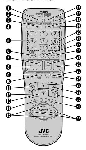
Buttons with a small dot on the left side of the name can also be used to operate your TV while holding down the TV button. F pg. 41
